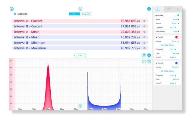
No. of independent interval analyzers 2 Jitter <20 ps Clock stability 500 ppb Digital resolution 1.95 ps Max interval rate 62.5 MHz Real-time and lossless
