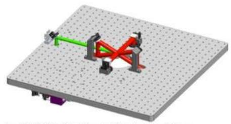
Level 3: 3D MOT, Optical Pumping & Imaging Beam Delivery Housing all beam preparation on the underside leaves plenty of space around the 3D MOT cell to mount user applications.
