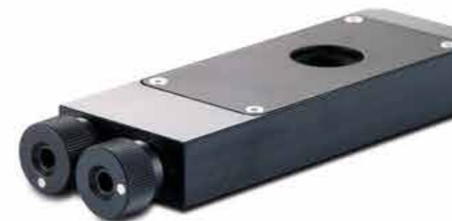
The holder for the phase plate was designed for easy exchange and simple alignment.
