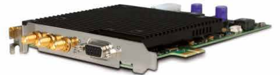
The TimeHarp 260 is a PCIe card type TCSPC electronics component with ultra short dead time. It is used for fluorescence as well as phosphorescence studies due to its extended range up to seconds.
