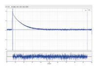
Time-resolved luminescence analysis of CIGS based solar cell. Measured with 20x air objective, excitation at 560 nm and emission detection at 1250 nm. The result of this analysis are three different decay lifetimes with 0.42 ns, 1.90 ns and 6.24 ns. This resulted lifetimes are strongly power depent, which is known in literature for this type of material.
