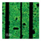
Fluorescence lifetime image of a CIGS based solar cell, 4x4 mm, 128x128 pixel, 1.1ms/pixel, excitation at 560 nm with LDH picosecond diode laser, detected emission at 1250 nm, nm, 40x air objective.
