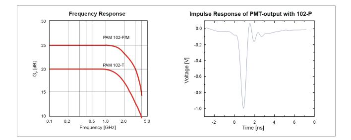
The PAM 102 pre-amplifier is specially targeted at timing sensitive applications such as Time-Correlated Single Photon Counting (TCSPC) with fast photon detectors like Microchannel Plate PMTs (MCP) or standard PMTs. Such detectors produce very small output pulses with extremely short pulse widths, usually too small for direct interfacing with TCSPC electronics or other counters.
