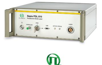
The Sepia PDL 810 system is a single channel pulsed diode laser driver system that allows operating a connected laser head in either pulsed or conitnuous wave (cw) mode. The driver may trigger the laser autonomously from its built-in crystal oscillator or, if a more complex triggering scheme is needed, can also be triggered by an external signal. Any output frequency from single shot (if triggered externally) to 80 MHz is supported.
