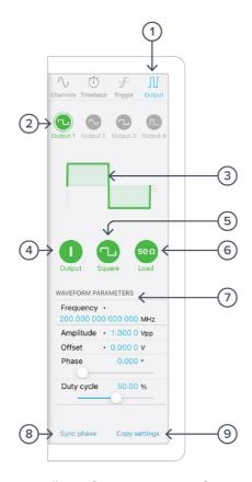
The output pane of the Oscilloscope allows for generation of various waveforms on Moku:Pro's output channels.
