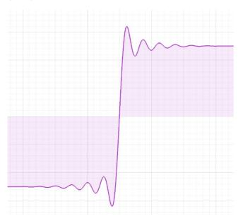
Also called "Sinc" interpolation, this mode preserves the frequency characteristics of the signal. In the time domain though, it can appear that there is over- or under-shoot that is not in fact present in the signal.
