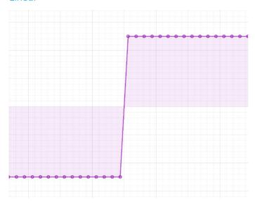
Linear interpolation does not perform any up-sampling. For display, it marks each point in the original data set and draws a straight line between them. This is "ugly" but doesn't "invent" any new data points.
