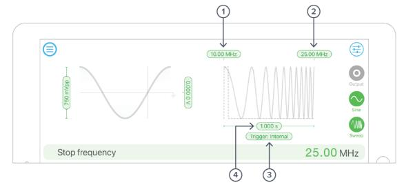
Sweep modulation acts like frequency modulation with a sawtooth, where the sawtooth starts on the trigger event.
