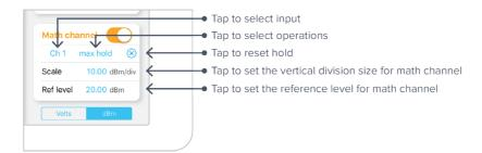
Four operations are currently supported by Moku:Lab's Spectrum Analyzer: +,  $\times$ , min hold, and max hold.
