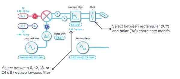
Rectangular (or Cartesian) coordinate mode measures the input signal with respect to a specific quadrature of the reference signal. When combined with a PID controller, Cartesian mode can be used to perform laser frequency stabilization.
