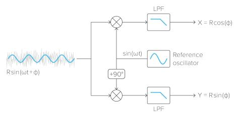
The demodulation process produces two spectral components: an *up-shifted* signal with a frequency equal to the *sum* of the input and reference signals, and a *down-shifted* signal with a frequency equal to the *difference* of the input and reference signals.
