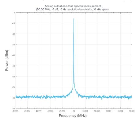
One-tone spectral measurement (50 MHz, -6 dBm, 100 kHz RBW, 500 MHz span)
