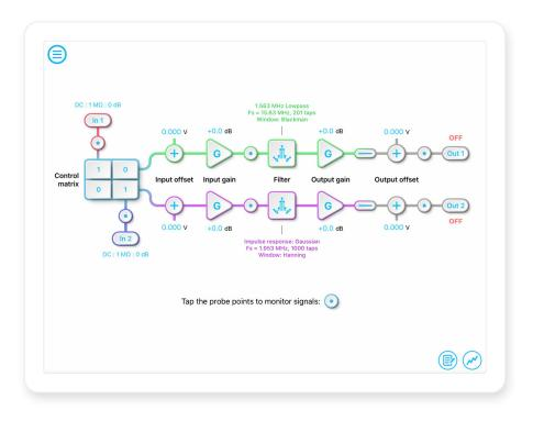
Sampling Rate<br/>Up to 15.625 MHzFilter Coefficients<br/>Up to 14,819Input Range<br/>± 0.5 V or ± 5 VOutput Voltage Range<br/>± 1 V into 50 ΩIntegrated Oscilloscope<br/>500 MSa/s
