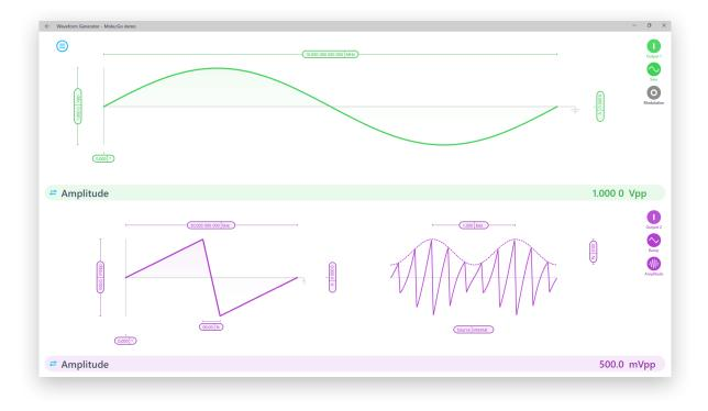
Frequency Range<br/>DC to 20 MHzSampling Rate<br/>125 MSa/sResolution<br/>12 bitOutput Voltage Range<br/>10 VppModulation<br/>FM, AM, PMOther Modes<br/>Burst, Sweep
