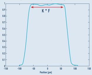
The Top Hat dimension is a function of the Top Hat constant (K) and is directly proportional to the focal/image plane of an optical system (F). Osela offers a wide variety of Top Hat constants and imaging lenses (F) to choose from, providing all the flexibility required for the most demanding Bioinstrumentation applications.
