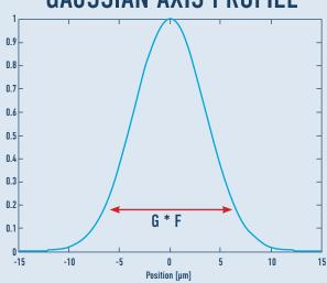
For the opposite Gaussian axis there are many options to choose from, providing great flexibility to the end user. The Gaussian axis is dependent on the focal length of the imaging lens system (F) and the G constant which is itself dependant on the model of the laser.
