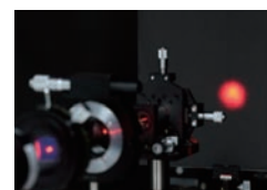
Intensity distribution when the pinhole diameter matches the focus spot
