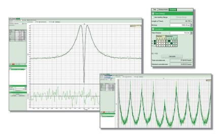
The QuCoa software package is an integrated solution for data acquisition and analysis using PicoQuant's TCSPC electronics in their unique T2 time-tagging mode. It is mainly targeted at all research areas that rely on coincidence detection such as Hanbury-Brown-Twiss setups to study single photon sources (g<sup>(2)</sup> / antibunching), quantum key distribution (QKD), or the study of entanglement using Hong-Ou Mandel (HOM) setups, to name only a few.
