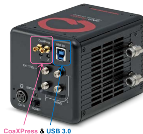
Figure 16. ORCA-Fusion can run through USB 3.0 or CoaXPress. The ORCA-Fusion was designed to be versatile and every ORCA-Fusion can be used with either USB 3.0 or CoaXPress. Since high speed imaging comes with additional costs and considerations, CoaXPress boards and cables can be added at the time of purchase or later as experimental needs evolve.
