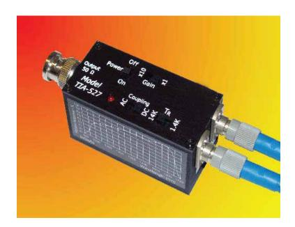
The TIA-527 balanced optical to electrical converter operates by subtracting the photo currents from two well-matched Indium Gallium Arsenide detectors. The result is then ampli ed and presented to the output port. Each of the optical signals causes the output to move with a different sense. Common mode signals (e.g. laser RIN noise) are effectively cancelled out.
