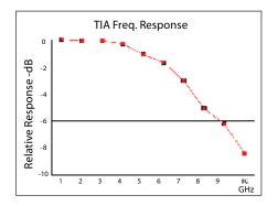
The TIA-4000 is comprised of a fiber coupled InGaAs APD detector combined with a variable reverse bias voltage network and fast transimpedance amplifier. The output of the unit brought out to a type K female SMA connector. Light falling on the detector generates a positive-going proportional current. This current, multiplied by the transimpedance produces a voltage that is proportional to the light incident on the detector surface.
