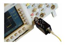
The TIA-1200 Optical to Electrical Converter is a wide-band detection system for fibre optic applications. With a typical bandwidth of DC to 14 GHz (min 12 GHz), it accurately provides an electrical replica of the optical signal presented to it. It is intended to drive a 50 ohm cable terminated in its characteristic impedance.
