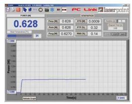
The Power mode permits measurements of laser powers with direct display of the actual value. The screen also shows the time evolution of power allowing stability measurements as long asseveral hours (up to 12 h depending on the PC).
