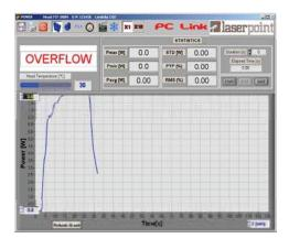
Every time the laser power or energy exceeds the head full scale an OVERFLOW alarm is displayed as shown in the picture.
