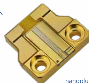
nanoplus high-power Fabry-Pérot laser on submount with AlN carrier
