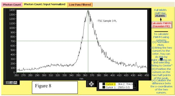
Note center wavelength of 364.2nm. Also note the small broad peak around 310nm. This is most likely an organic contaminant on the wafer piece. Further evaluation shows it is most likely finger print containing Tryptaphane.
