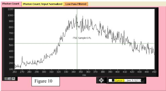
Note that again the PL is not as intense as in other runs. There is also a large and slow decaying tail toward the Red side of the spectra. Note there is also a Raman Peak at the 3200cm-1 area of the spectra. Most likely this is bound water in the wafer. I do not know why this sample has so much water, maybe it is Hydroscopic in nature.
