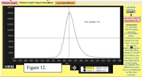
Note this sample has the highest PL output and a very crisp peak with a FWHM  $\sim$ 22.3nm The center wavelength is  $\sim$ 358.4nm.
