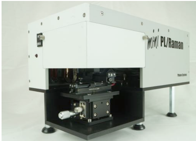
Mini PL 110 with optional X-Y motorized stage
