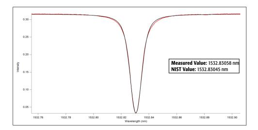
Wavelength data (red) measured with the model 871A-NIR as a laser tunes through an absorption of acetylene gas (NIST SRM 2517a). A Voigt curve fit of this data (black) gives a measured absorption wavelength of 1532.83058 nm. The published NIST value of 1532,83045 nm is well within the wavelength meter's accuracy of  $\pm$  0.3 pm.
