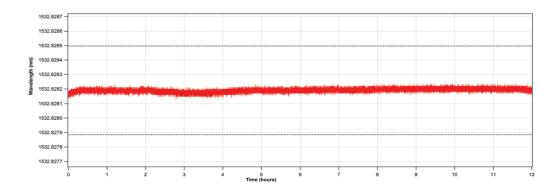
Long-term wavelength measurement data of a DFB laser locked to an absorption line of acetylene. The specified accuracy is given by the dashed lines.
