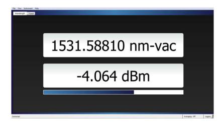
The IR and MIR versions of the model 671 do not measure optical power, and therefore only display wavelength measurements and a graphical respresentation of relative intensity to aid with instrument alignment.
