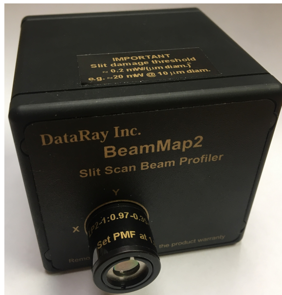
Figure 1: A scanning slit device mounted with a LensPlate2. LensPlate2 reimages the beamwaist onto the zero plane of the detector that lies within the beam profiler's case. The magnification is marked on the unit.
