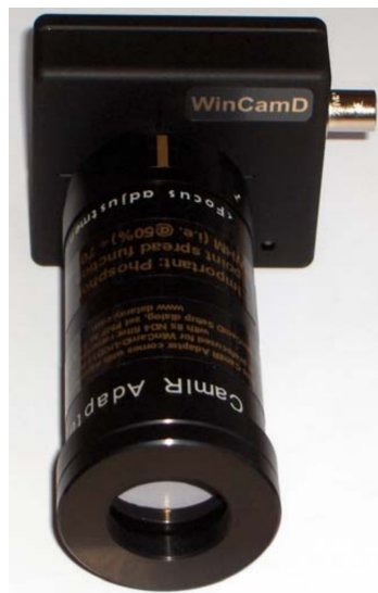
Figure 1: The CamIR adapter correctly attached and focused - ready for use
