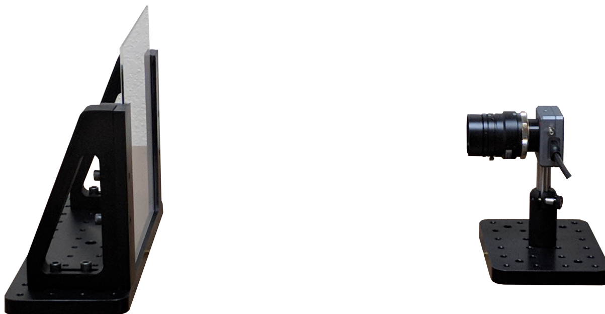
Figure 1: WinCamD-LCM with lens reimaging a transmissive diffusing screen.
