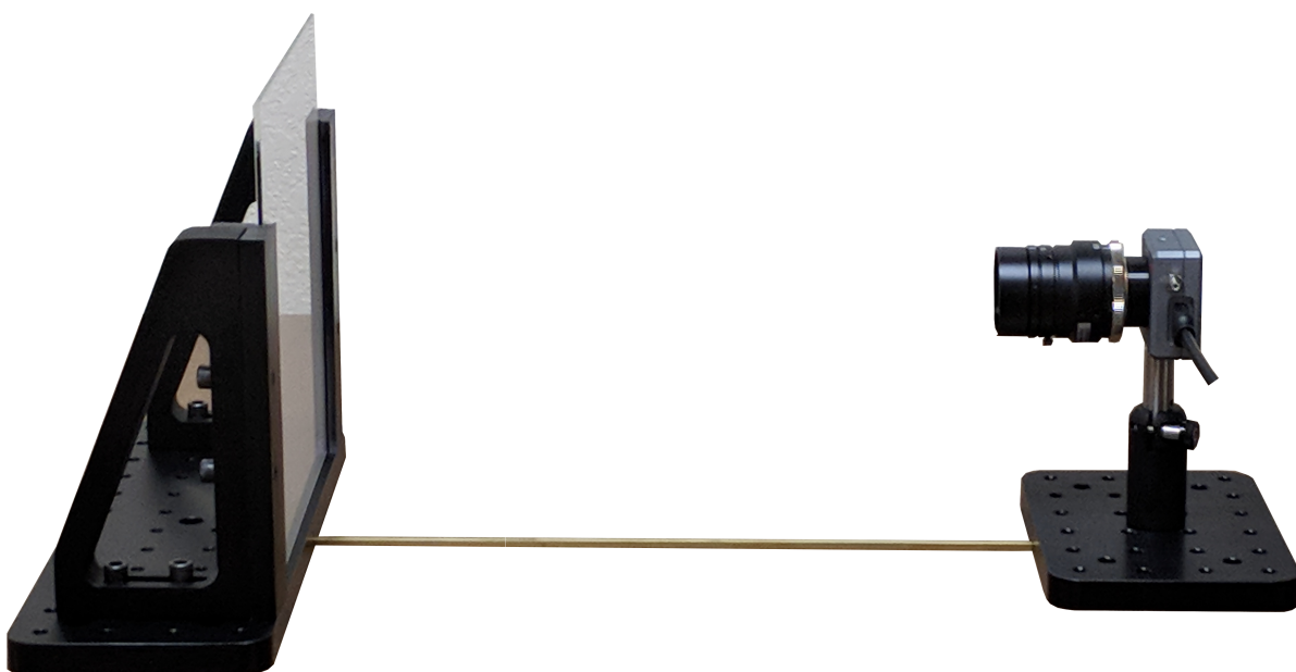
Figure 2: The camera is pre-calibrated for the setup shown above. If a different object distance is used, the PMF must be recalibrated (See Appendix A)
