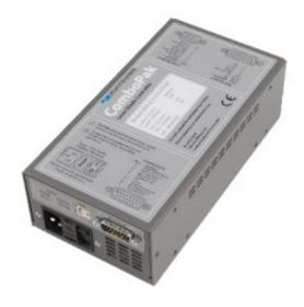
The 685-02 ComboPak offers excellent laser performance for pump lasers, higher power LEDs, and other devices requiring up to 2A of drive current. With 100uA set point resolution and less than 40uA of noise, the 685-02 provides a transparent driver that won't interfere with the performance of your laser or LED devices. Couple that with a high performance TEC controller that supports excellent long term stability and high resolution.
