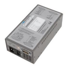
The **685-01 ComboPak** offers excellent laser performance for pump lasers, higher power LEDs, and other devices requiring up to 1A of drive current. With 20uA set point resolution and less than 50uA of noise, the 685-01 provides a transparent driver that won't interfere with the performance of your laser or LED devices. Couple that with a high performance TEC controller that supports excellent long term stability and high resolution.
