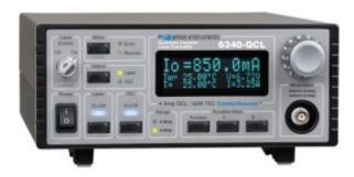
The **6340-QCL Quantum Cascade Controller** is designed for quantum cascade lasers (QCLs), which operate at a much higher voltage than typical laser diodes, providing up to 15 voltage of compliance. Combine that with excellent current performance, with both a 4 Amp and 2 Amp operating range, as low as 100uA set point resolution and less than 40uA of noise, the 6340-QCL provides a transparent driver that won't interfere with the performance of your quantum cascade laser .
