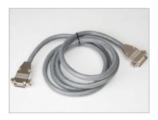
Similar to the 1260B TECSource Cable, but adds wiring for 4-wire RTD configuration, and also support for operation up to 10A. The cable is terminated with DB-15 connectors on both ends for quick connection to any Arroyo Instruments mount.
