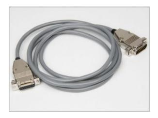
Our standard TECSource interconnect cable. This cable is good for applications up to 5A and includes wires for the fan connection. The cable is terminated with DB-15 connectors on both ends for quick connection to any Arroyo Instruments mount.
