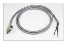
The 1233 is a 40A-rated cable for use with high current instruments. The cable is terminated with a 13W3 male connector on the instrument end and bare wires on the mount end.
