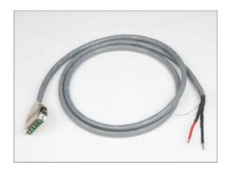
The 1229C is a 20A-rated cable for use with the 4320 and other high current instruments. The instrument end as the standard 9W4 connector, while the mount end of the cable has unterminated tinned wires for connections to custom mounts.
